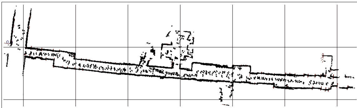
Fig. 7. Laser scans overlaid on SLAM map using corrected robot path.
